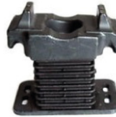
PRS 6021 MOTOR TAKOZU ENGINE MOUNTING CF75 - CF85 - XF105 - XF95 OEM KODU / OEM CODE : 1779767 FİYAT / PRINCE : 1699564
